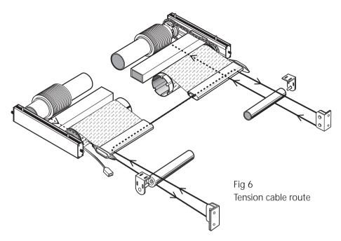
Attach the cable to the outer end of the cable drum where there is a clamp. Now pull sufficient cable off the reel so that the wire can be cut and attached to the other cable drum. Leave a small amount of slackness in the wire so that when the tension is taken up there will be a minimum of one turn of cable on the each drum. Note that the cable will centralize itself around the hem-bar pulley.
