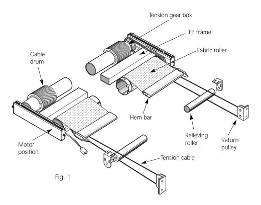
This manual describes the installation, method of operation and maintenance for the double roller tension blind system type TESS 200. The TESS 200 system comprises an aluminium H-frame containing two rollers which are coupled together. One roller carries a fabric or screen and the other roller has two cable drums to take up a wire which is attached to the hem-bar on the end of the fabric so that the fabric can be drawn under tension across a horizontal or vertically sloping glazed structure.
